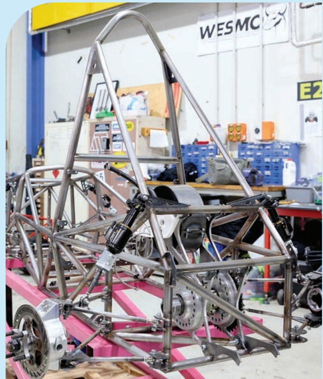
Formula SAE race car space frame fabricated from UltraTube RS by the University of Waikato's WESMO team.
